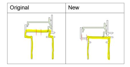
The new frame profiles for DGS F30Z with **flange width 28** also use a **new corner cleat: G0100797**! The frame profiles, with flange widths 24 and 32 continue to use the usual clamping angle.
