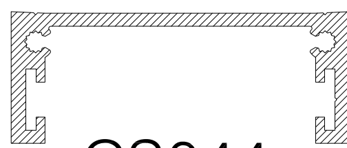
CS044 25mm SLIDING DOOR FRAME HEAD OR JAMB
