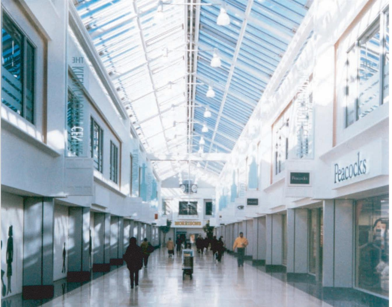
The T-shaped covered mall is a two-storey complex with the supermarket covering gross floor area of 83,185 sq ft. The 35 retail units cover a gross area of 100,00 sq ft on two floors. The flexibility and integration of Comar Aluminium Systems can be appreciated within this project. Profiles from 8 systems integrate to provide roof glazing, curtain walling, windows, door and ground floor treatment solutions.
