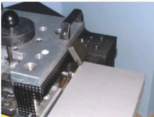
Plate. 6. Slide rails between dies (107 and 108).
