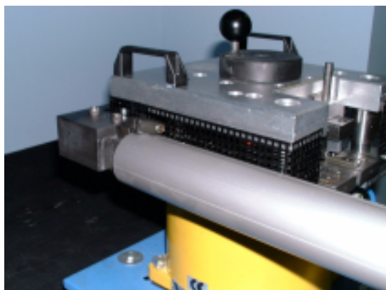
Plate 1. Engage the dovetails into the punch tool, up to the pre-determined stop.
