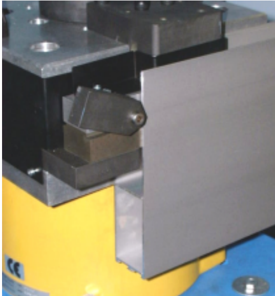
Plate 9. Punching rail to accept bottom pivot – 70mm pivot point for 55mm stile shown.
