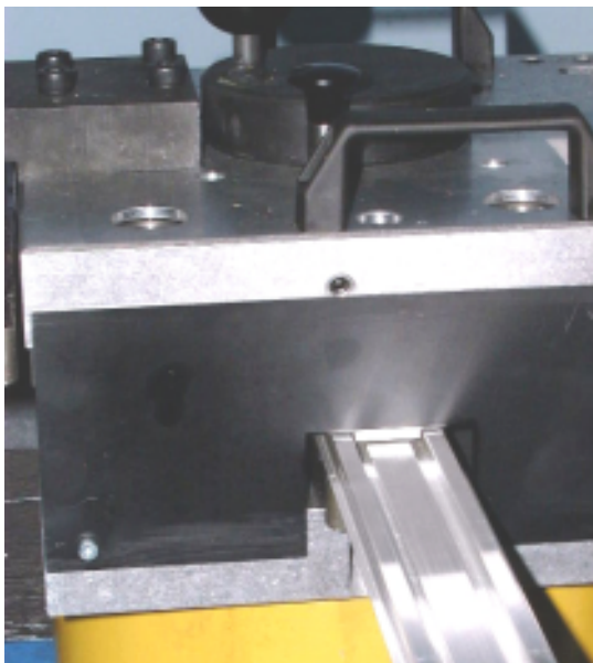
Plate 10. Insert brush carrier face down locating the dovetail.
