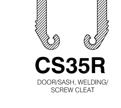
CS35R DOOR/SASH, WELDING/ SCREW CLEAT
